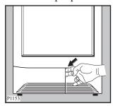
During the drying cycle or at the end, it is normal for water to be present on the surface of the condenser insertion.
